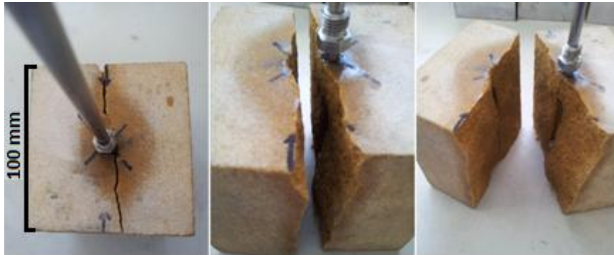
Figure 5: Figure 5: View of sample two after HF test: the fracture opened along the maximum stress direction.
