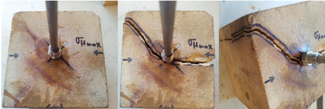
Figure 5-6 View of sample one after HF test; one fracture wing (on the left) was not propagated along the maximum stress direction.
