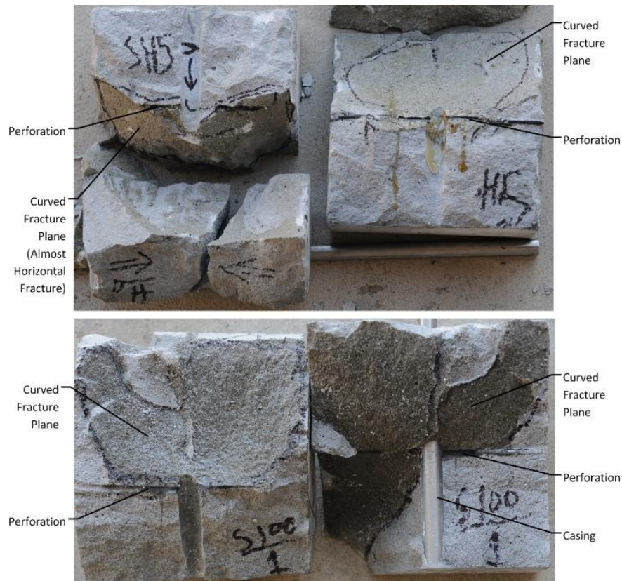
Figure 5-14 Fracture geometries of tests H-4 (top) and SL-1 (Bottom).
