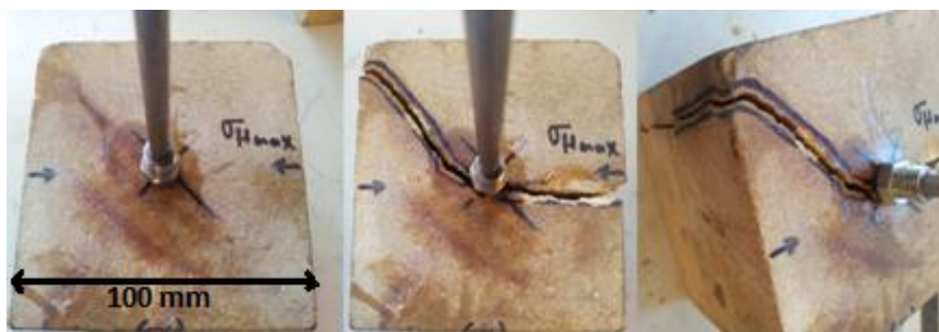
Figure 3: View of sample one after HF test: one fracture wing was not along the maximum stress direction.
