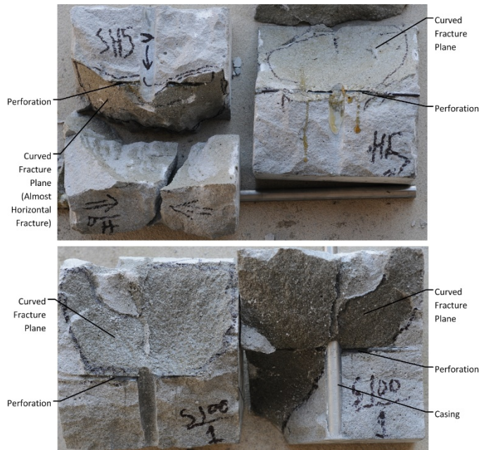
Figure 8: Fracture geometries of tests H-4 (top) and SL-1 (Bottom).
