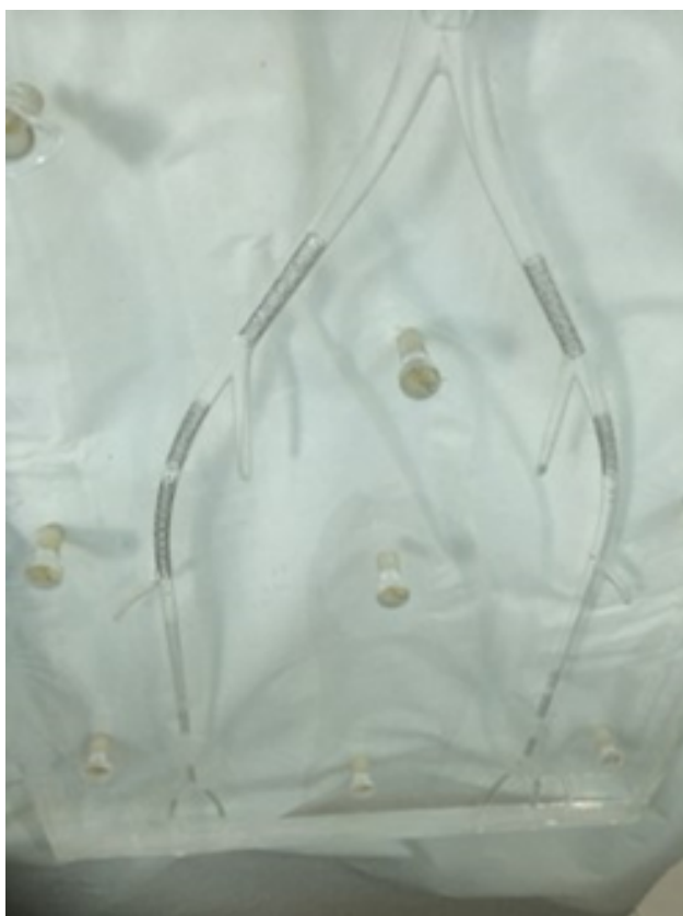
Figure 4.1. Photograph of the phantom with stent insertions
