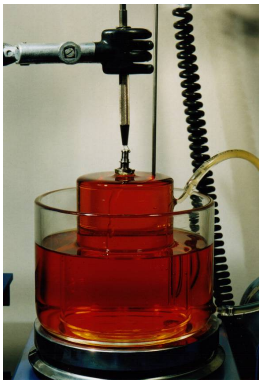
Figure 3.2: Temperature controlled overflow cell containing ferric sulphate solution in contact with chalcopyrite massive sample.
