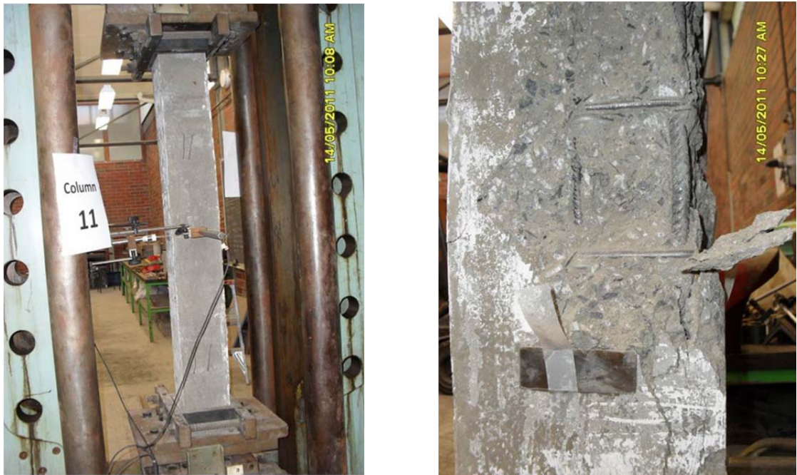
Figure 4.11: Failure mode of column GCIV-C2: (a) column after failure; (b) closer view of failure section
