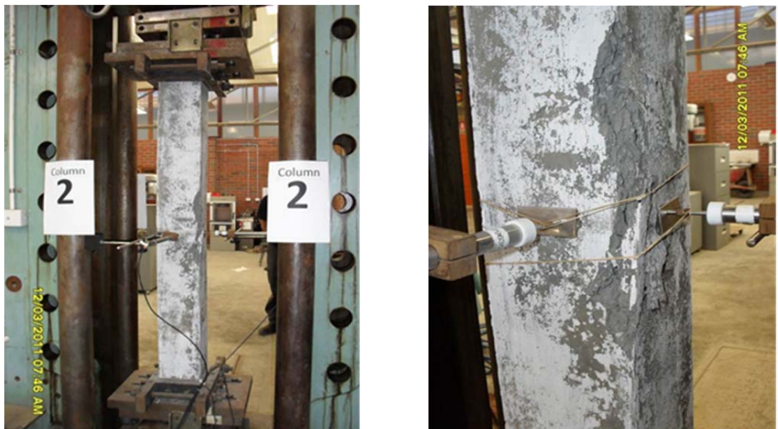
Figure 4.2: Failure mode of column GCI-C2: (a) column after failure; (b) closer view of failure section
