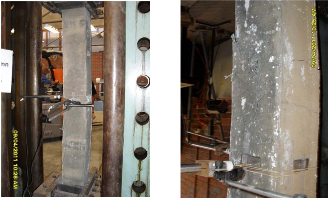
Figure 4.3: Failure mode of column GCI-C3: (a) column after failure; (b) closer view of failure section
