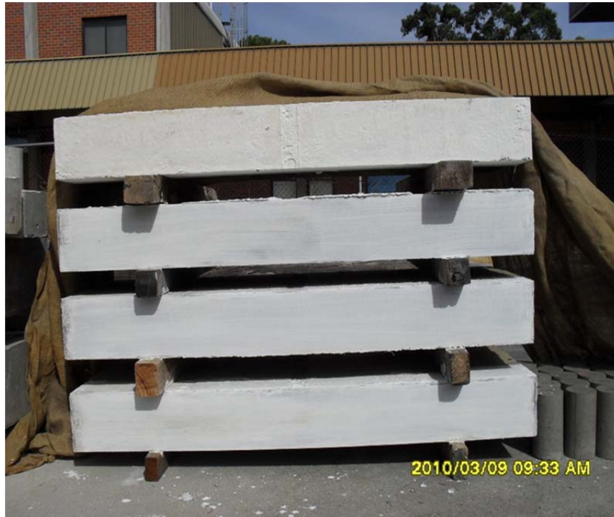
Figure 3.8: Test columns and cylinder specimens after steam curing
