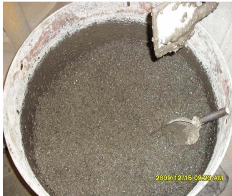
Figure 3.4: Fresh Geopolymer Concrete
