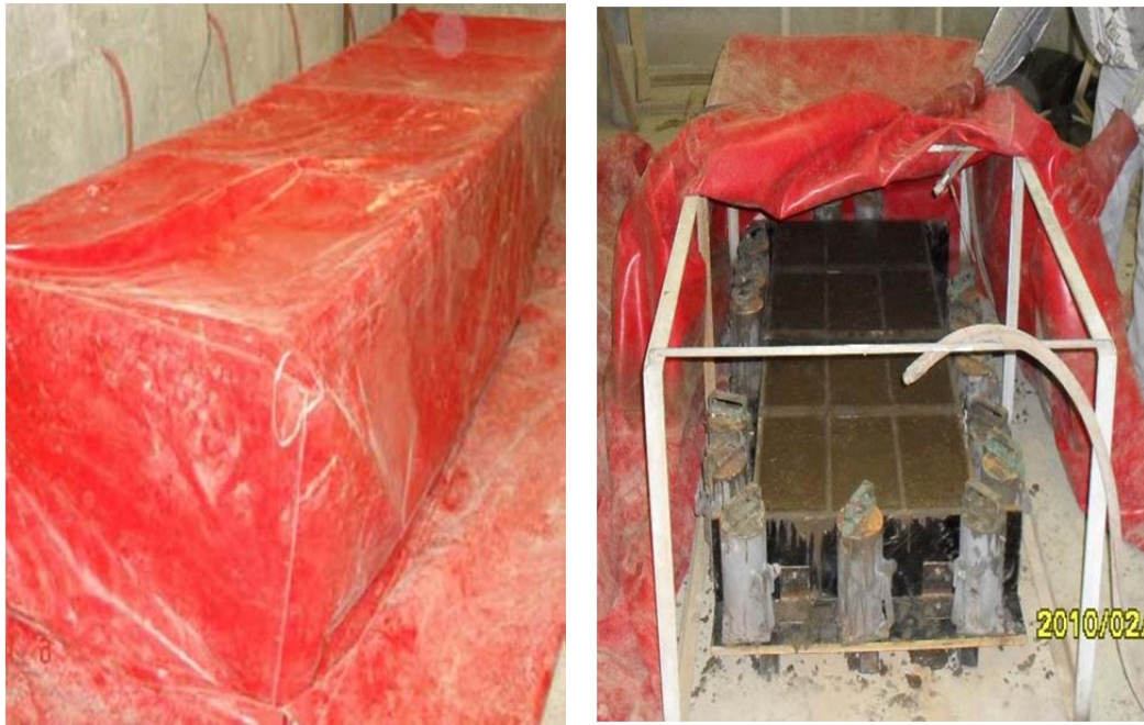
Figure 3.6: Set-up of Steam Curing Chamber
