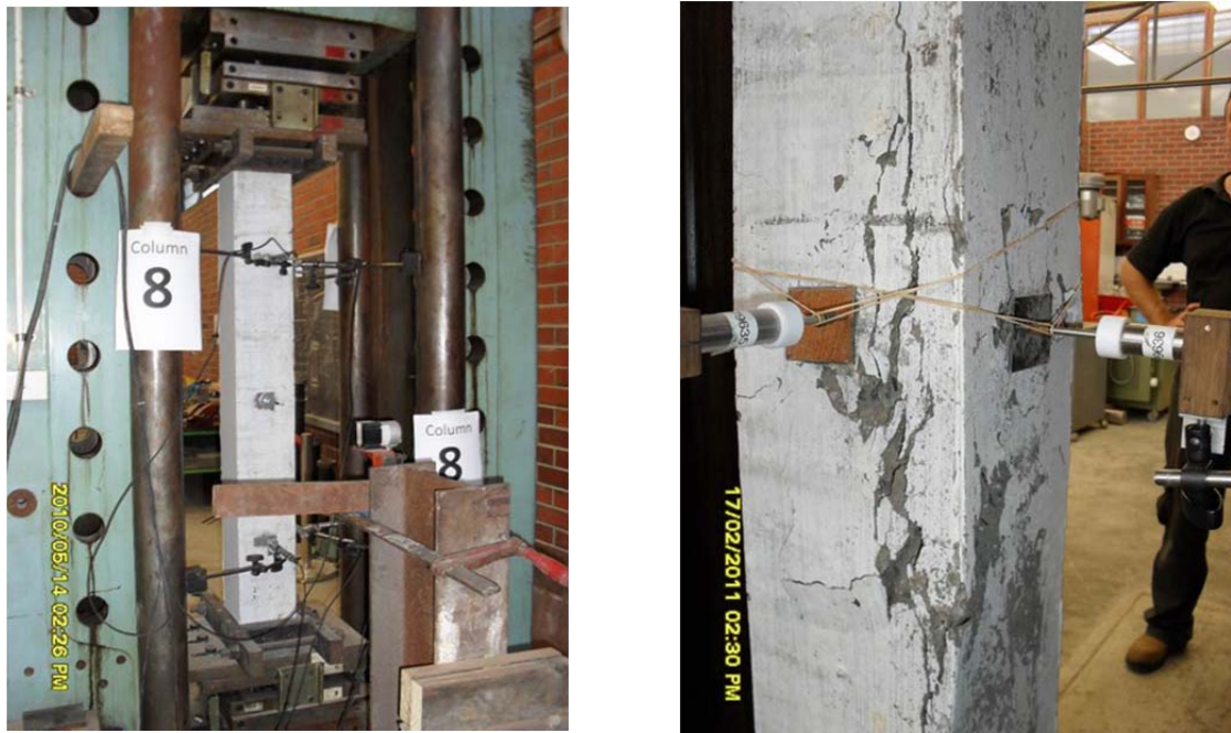
Figure 4.8: Failure mode of column GCIII-C2: (a) column after failure; (b) closer view of failure section
