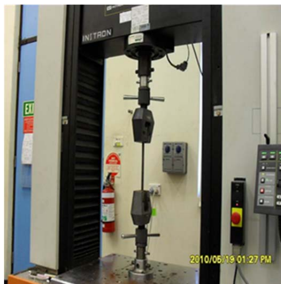
Figure 3.1: Test of reinforcing steel
