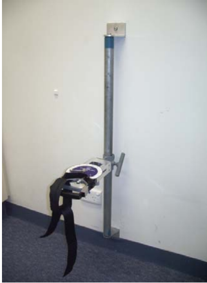
Figure 3.8 (A-C) Wall-attached dynamometer and the procedure of knee strength tests.
