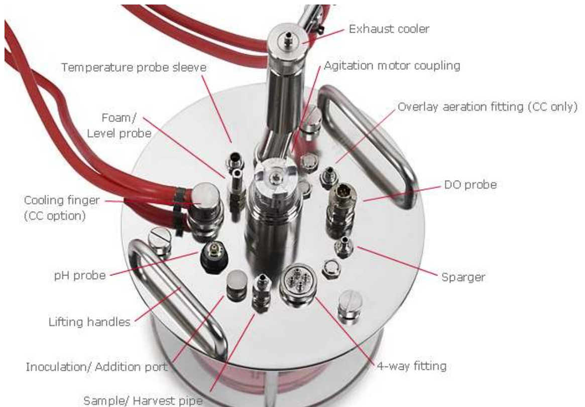
Figure 3-3 Bioreactor Top Plate
