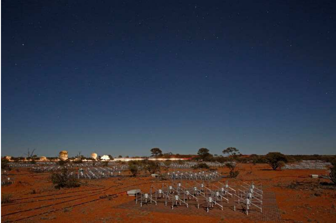
Figure 2.8: A photograph of the MWA antenna tiles, with analog beamformer seen as a box on each of the tiles. Each tile (a 4 x 4 dipole array mounted on a 5 x 5 m wire mesh) is laid directly on the ground, with 16 dipoles clipped onto the mesh (credit: Chris Thorne).
