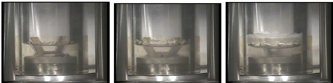
Figure 21: Hydrate growth trend 1000ppm at 50bar
