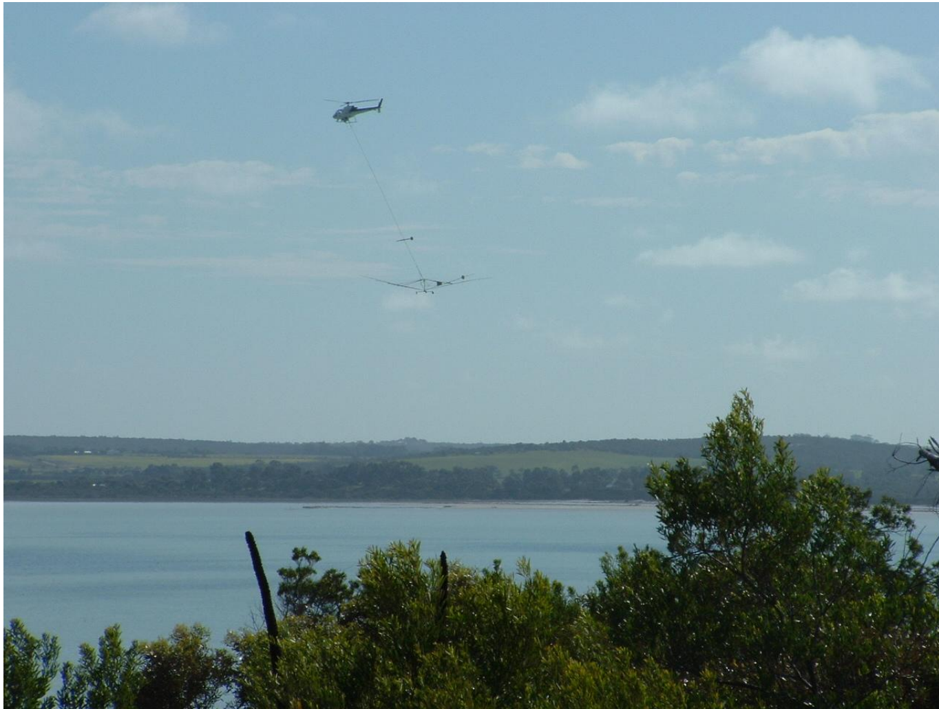
Figure 46. HoistEM surveying over Pink Lake.
