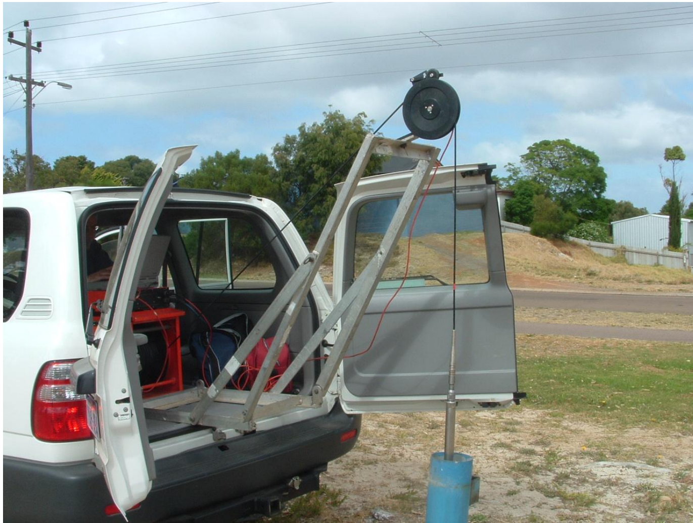
Figure 60. EM39 down-hole logging at Esperance.
