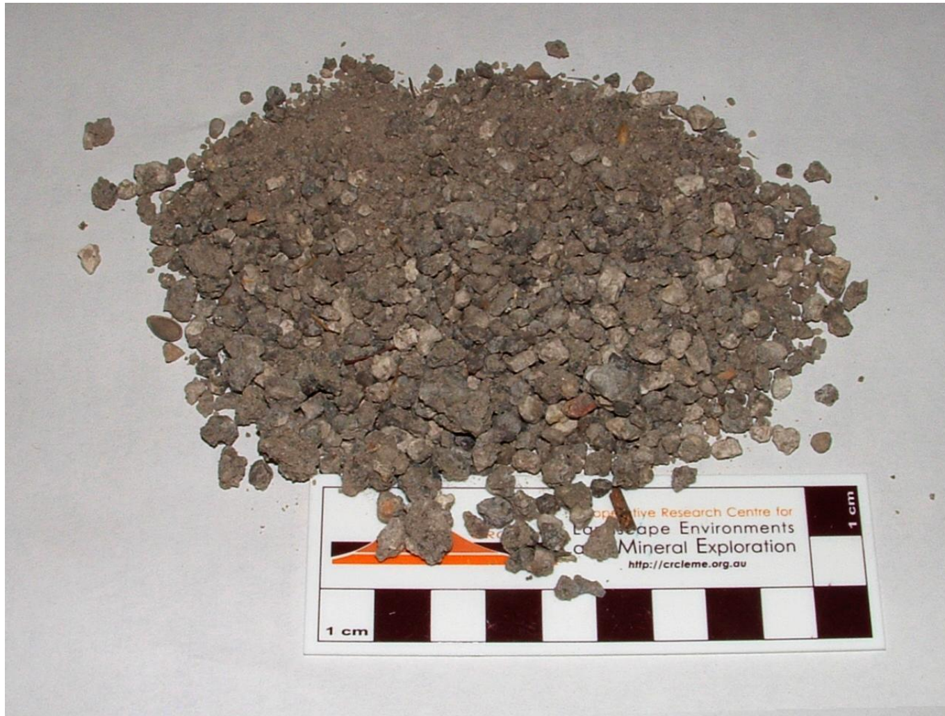
Figure 32. Material retrieved from below 41m in the production bore during drilling.
