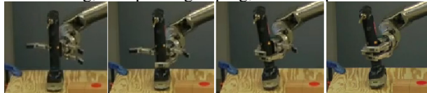
Fig. 8: Steps for drill grasping using compliant manipulation: touch shaft, touch base, capture shaft, and actuate the button.
