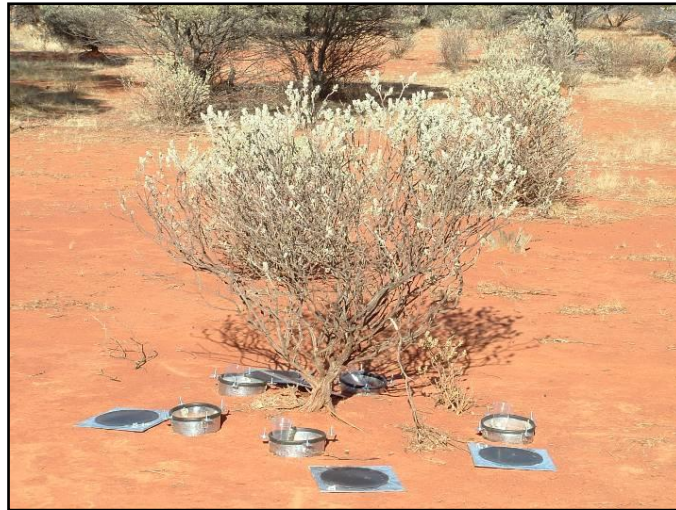
Plate A-1: Five respiration rings partly installed at a P6 shrub patch
