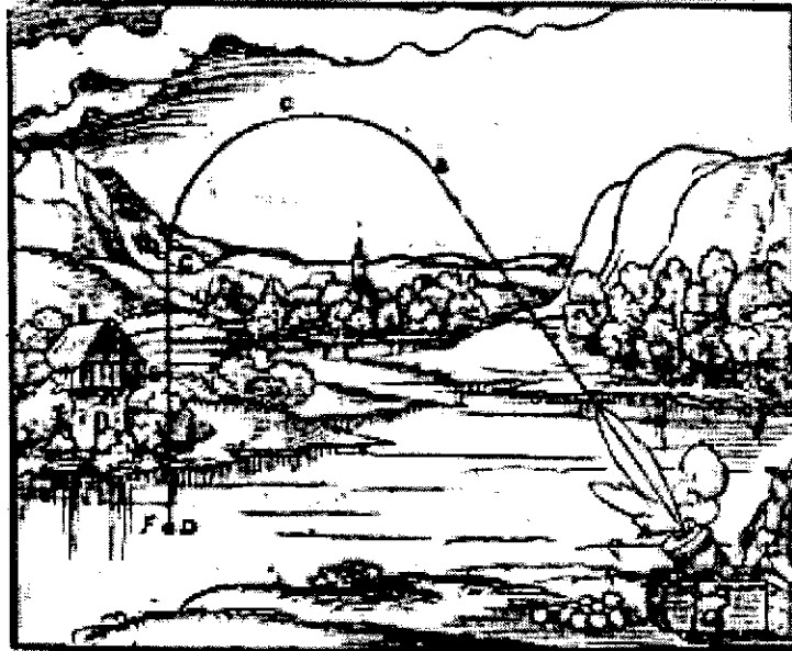
Figure 3.4. This drawing is reproduced from the 1582 edition of Baukunst Oder Architectur aller furnemsten , by Walther Ryff. It illustrates a version of the impetus theory that divides the trajectory of a projectile into three phases. In the first phase, the impetus provided by the canon overpowers the weight of the object and the projectile moves in a straight line. The impetus gradually dissipates and its weight causes the projectile to begin to curve downwards. In the second phase the projectile’s movement is influenced by the impetus of the canon and the downward impetus imparted by its weight. In stage 3 the impetus is zero and it falls straight down (from McCloskey, 1983a, p. 114B).
