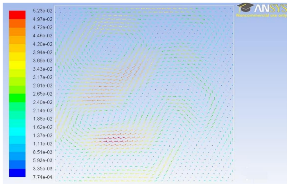
phase-2-velocity Colored By Velocity Magnitude (phase-2) (m/s) (Time= 2.0700e+02) Jun 18, 2016 ANSYS FLUENT 14.0 (2d, dp, pbns, eulerian, spe, lam, transient)
