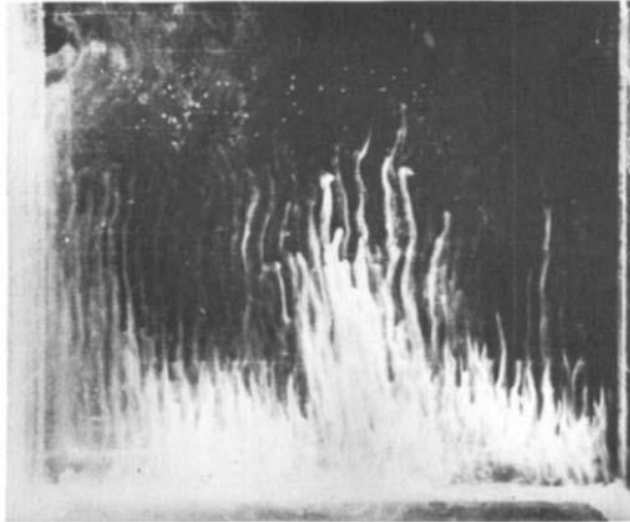
Figure 2.1: Vertical cross section of salt fingers (diffusion fingers) 36 .
