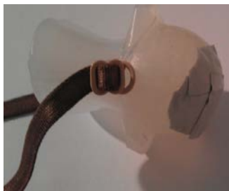
Fig. 3. Silicone tongue device with attached reflective tape
