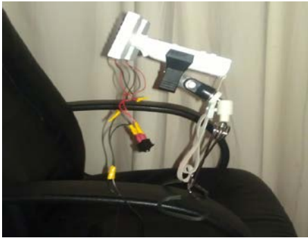
Fig. 6. Mounting the TACS to a chair using a clamp
