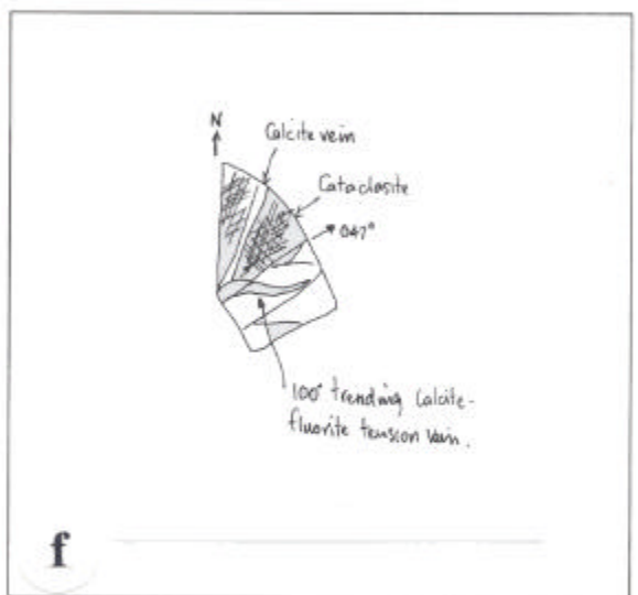
Figure 5.6 - a) Typical cataclastic fault zone in dolerite. b) Cataclastic texture in bleached dolerite c) Photomicrograph of cataclastic texture in pyrite, reflected light. d) Photomicrograph of chloritic microfault cross-cutting cataclasite, (XPL). e) Same view as in d), (XPL). f) Sketch of hand specimen showing microfaults and late granitoid related veins cross-cutting cataclasite. See text and over page for explanation.
