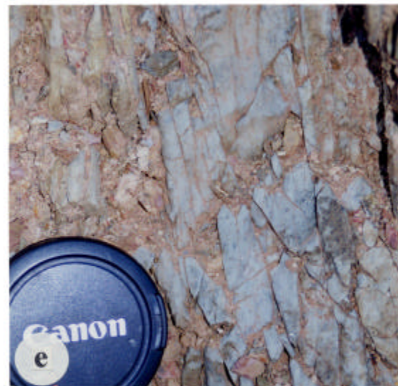
Figure 3.6 - a) Porphyry / ultramafic contact, Anthill open-pit. b) Type II S-C mylonite, Bowerbird diamond drill core. c) Zuleika Shear Zone in weathered basalt from Bullant open-pit. d) Zuleika Shear Zone in fresh basalt from Bullant open-pit. e) Multiple brittle fractures in schistose basalt, Bullant open pit. f) Line drawing of Figure 3.6e. See text and over-page for explanation.
