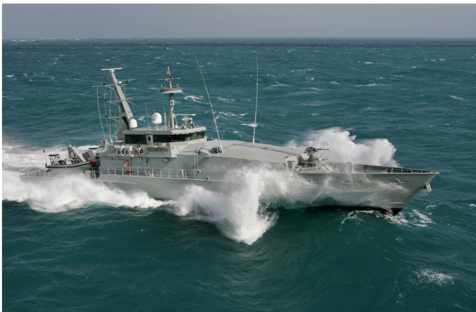
Figure 1.1 – A 56.8 m Armidale class patrol boat is known to have excellent seakeeping qualities despite experiencing hull bottom slamming in rough seas (photographs courtesy of Austal, Australia, 2010).
