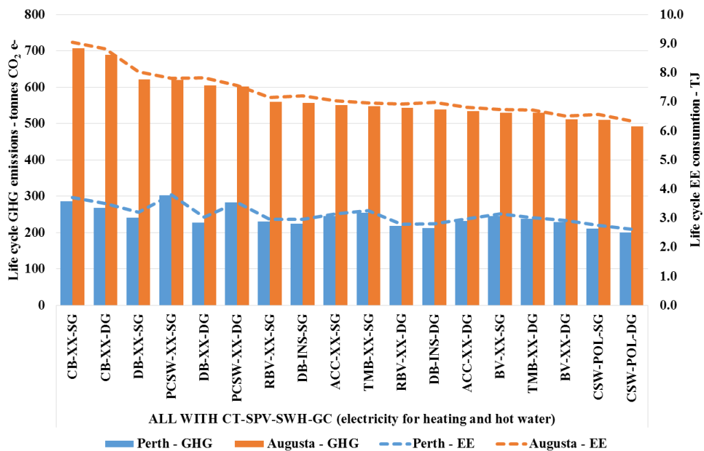
Figure 6.8 Comparison of life cycle GHG emissions and EE consumption of all CPS options between Augusta and Perth (use of electricity for heating and hot water)
