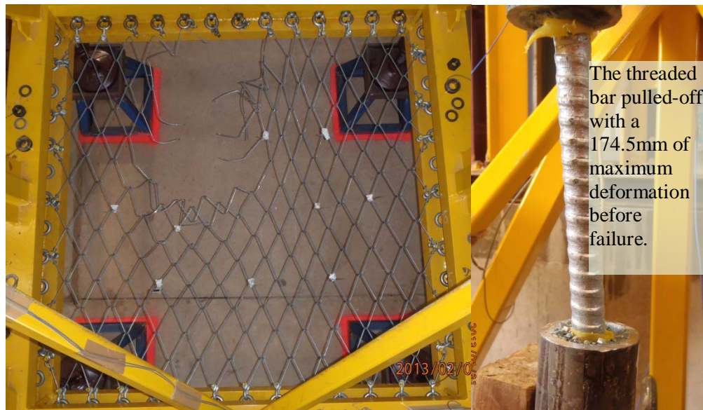
Figure 99: Post-test setup of sample 200
