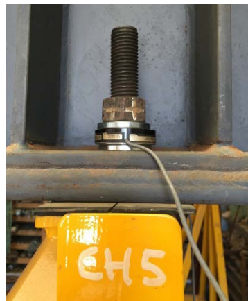
Figure 25: Load cell between the drop beam and mesh frame attachment.
