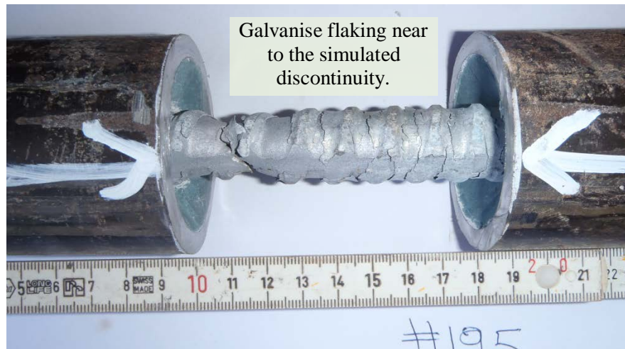
Figure 85: Displacement at the simulated discontinuity
