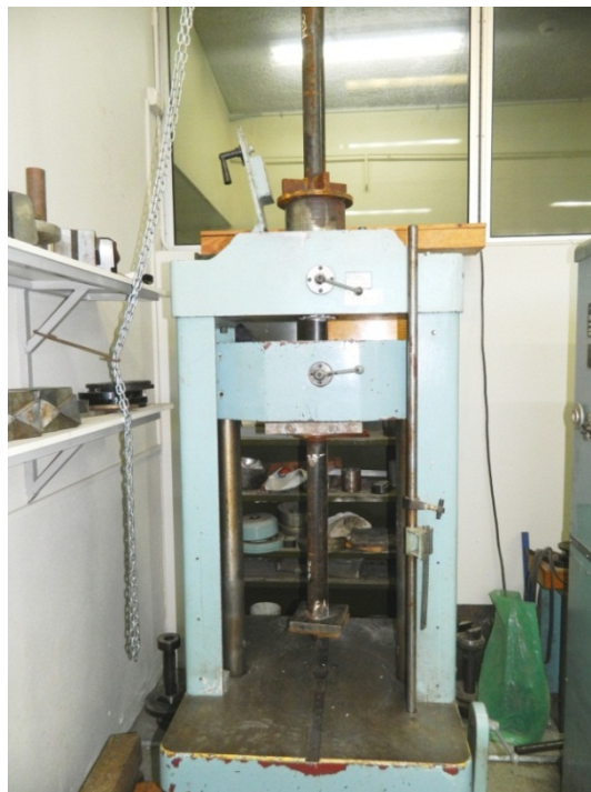
Figure 37: Static test setup for reinforcement
