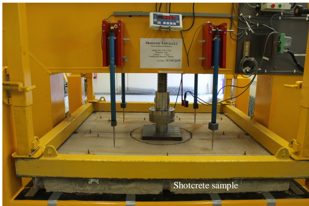
Figure 39: The configuration of WASM static test facility for shotcrete testing (Morton et al., 2007).
