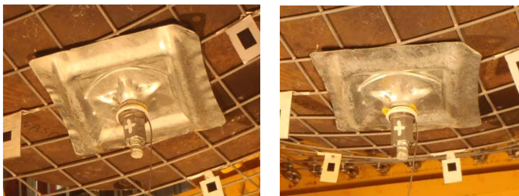
Figure 82: (L) Pre-test and (R) Post-test surface hardware of sample #197.
