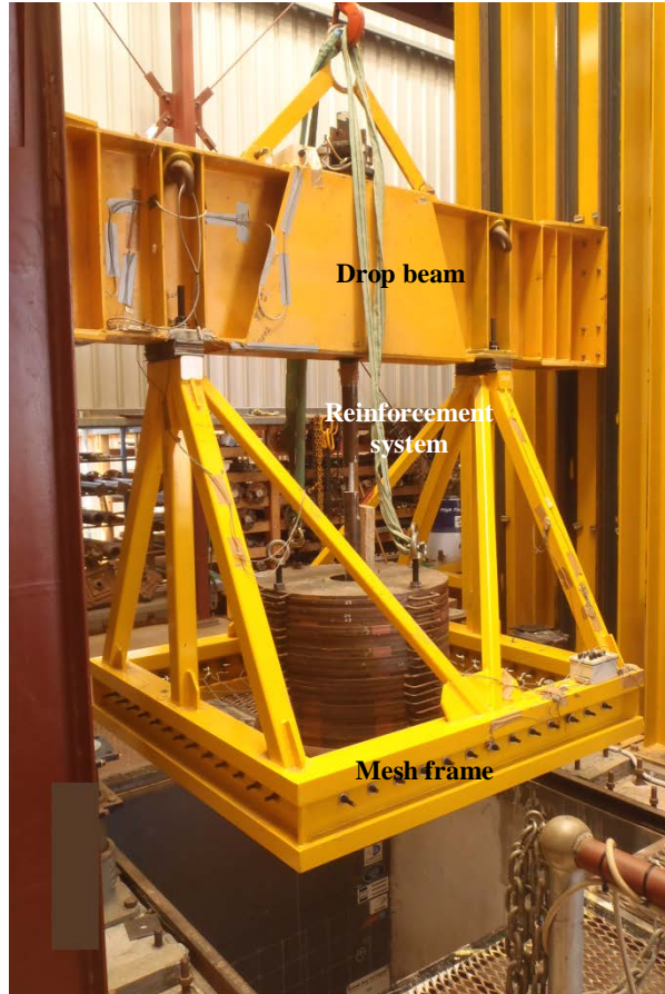
Figure 52: Lowering down the system onto the buffers.
