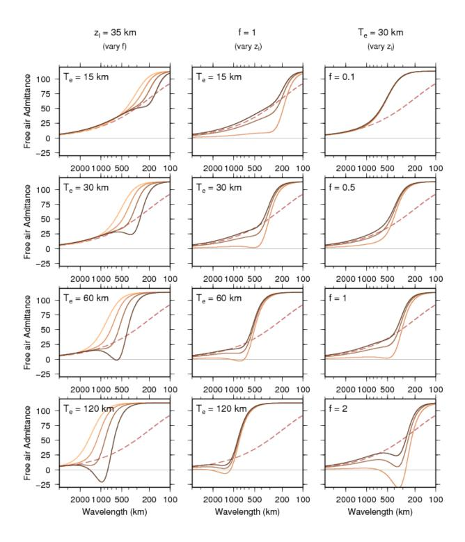
Fig. 1. Theoretical free air admittance curves for various indicated values of  $T_e$ , f and depth to internal load ( $z_l$ ), where f is uniform, i.e., has the quoted value at all wavenumbers. The shading of the curves gets darker as the quantity increases. In the left-hand column (constant  $z_l$ ) the curves show the variation with f = 0.1, 0.5, 1 and 2. In the middle column (constant f) the curves show the variation with  $z_l = 10, 25$  and 35 km. In the right-hand column (constant
