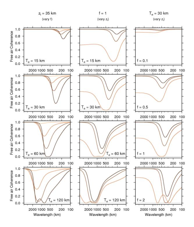
Fig. 3. Theoretical free air coherence curves for various indicated values of  $T_e$ , f and depth to internal load  $(z_l)$ . The shading of the curves gets darker as the quantity increases. In the left-hand column (constant  $z_l$ ) the curves show the variation with f = 0.1, 0.5, 1 and 2. In the middle column (constant f) the curves show the variation with  $z_l = 10, 25$  and 35 km. In the
