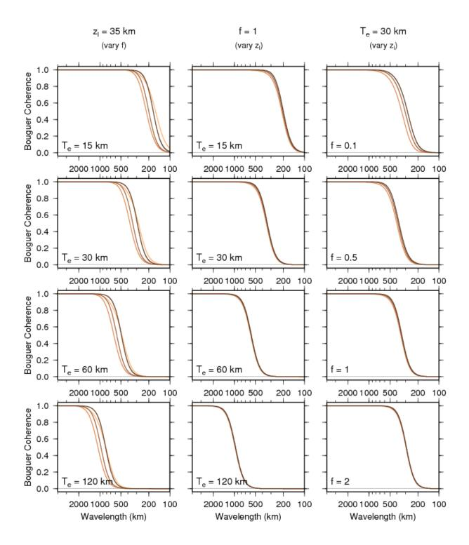
Fig. 2. Theoretical Bouguer coherence curves for various indicated values of  $T_e$ , f and depth to internal load  $(z_l)$ . The shading of the curves gets darker as the quantity increases. In the left-hand column (constant  $z_l$ ) the curves show the variation with f = 0.1, 0.5, 1 and 2. In the middle column (constant f) the curves show the variation with  $z_l = 10, 25$  and 35 km. In the
