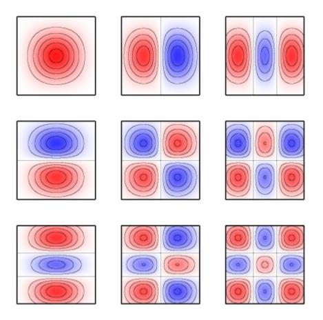
Fig. 5. The 9 2D Slepian tapers in the space domain corresponding to a bandwidth parameter of NW = 2. The data are multiplied by each taper and then Fourier transformed, giving 9 estimates of the data's power spectrum; these are then averaged to give the power spectrum of the data. Red colours are positive, blue negative.
