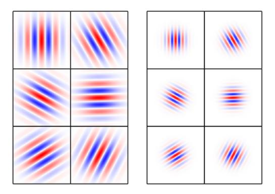
Fig. 7. The real part of 6 2D Morlet wavelets in the space domain at large (left) and small (right) scales, each at a different azimuth (imaginary part not shown). The data are convolved with the wavelets at many scales, and scales are mapped to wavenumber. The convolution yields wavelet coefficients as functions of space, wavenumber and azimuth; their modulus-squared gives the wavelet power spectrum. Red colours are positive, blue negative.
