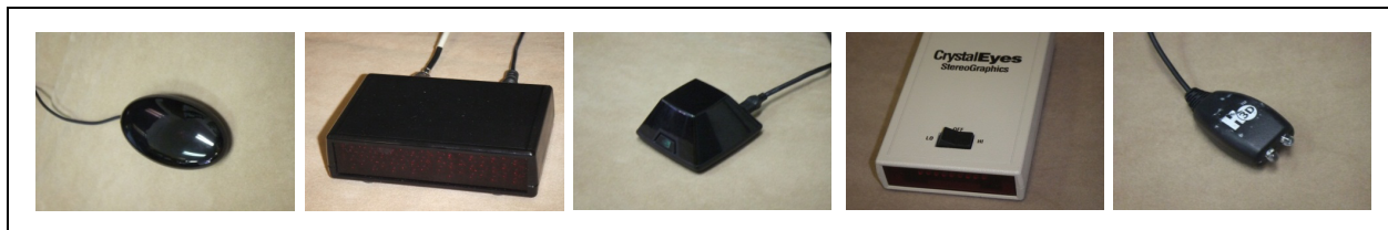
Figure 2: Some of the stand-alone IR 3D emitters tested: (a) Samsung 2007, (b) NuVision, (c) NVIDIA 3D VISION, (d) CrystalEyes 1, and (e) H3D/ELSA.
