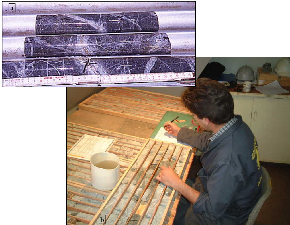
Figure 2.16. - Standard un-oriented core samples, prior it is split (a) and after that (b).
