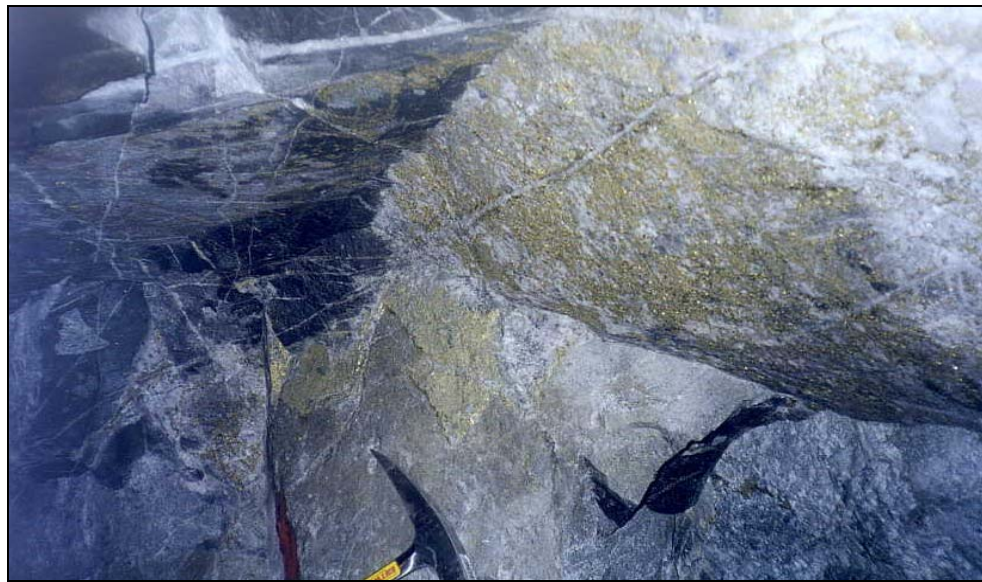
Figure 2.7. Mine wall at the El Teniente mine, showing how vein infill and alteration may cover the rock exposure, sometimes hiding structural data behind.
