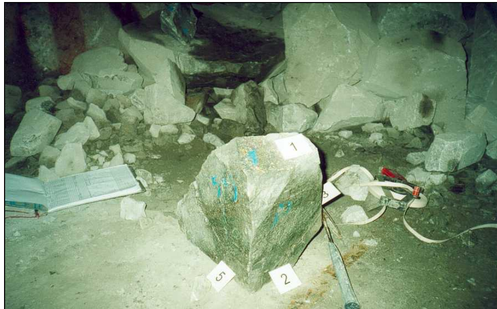
Figure 2.21.- Characterised rock block showing trapezoidal prismatic shape in a draw point at the Reno mine sector (Figueroa, 2003).
