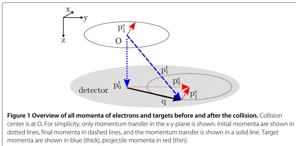
Momentum in x- and y-direction can be calculated from the impact position of the excited target on the detector and its time-of-flight  $t_f$ :
