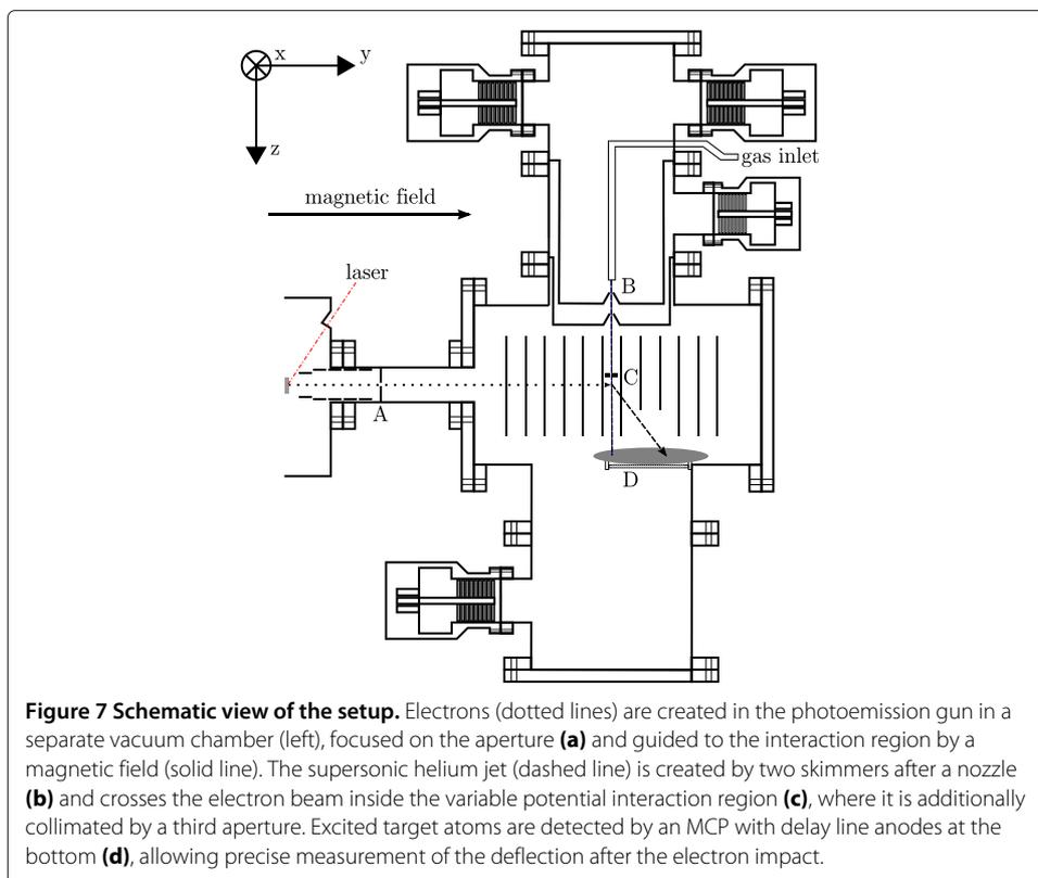
is 3 K. With this setup a beam diameter of about 2 mm and a target number density of  $1.5 \times 10^{11} \text{ cm}^{-3}$  can be obtained in the region of interaction with the electron beam. To increase resolution, the beam is additionally collimated by inserting a 500  $\mu\text{m}$  aperture a few millimeters above the interaction point, which is held at the same potential as the surrounding region at all times. The beam is dumped directly into the chamber without an additional dump stage.
