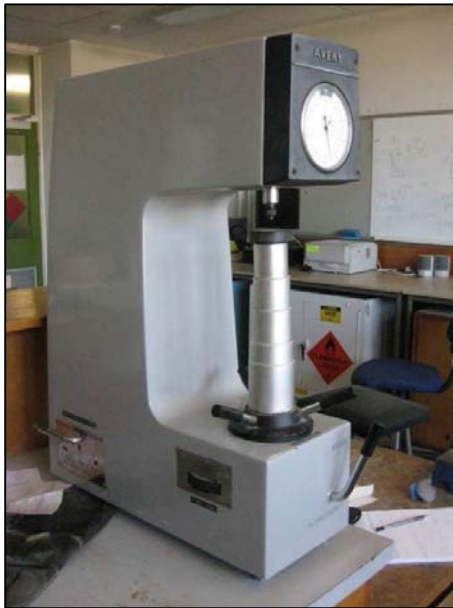
Figure 3.2: Avery Rockwell hardness tester.
