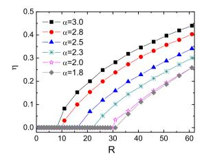
FIG. 1: (Color online) The order parameter  $\eta$  versus R for weighted scale-free networks with different routing parameter  $\alpha$ . Other parameters are networks size N=1000, m0=m=5, W=2 and  $\beta=1$ .
