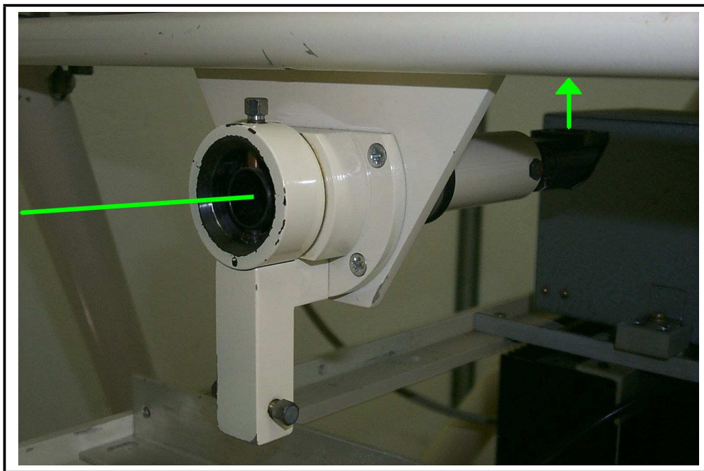
Figure 4.5: The adjustment screws used to position prism M4.
