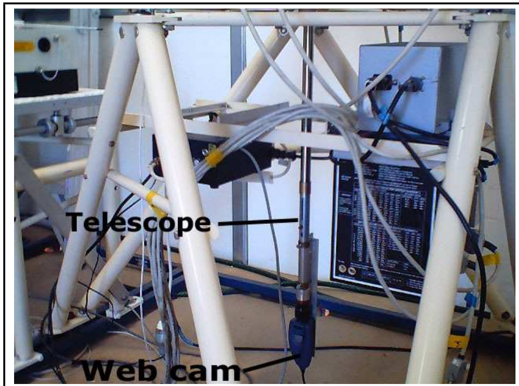
Figure 4.11: This image shows the camera, almost on the floor, looking up through the laser output optical system.
