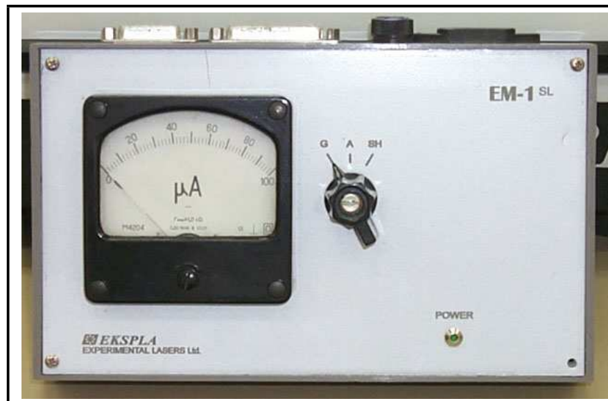
Figure 5.15: Comparative energy meter used with the SL212 laser. The selector switch on the right can be set for G - generator, A - amplifier or SH - second harmonic (final output).
