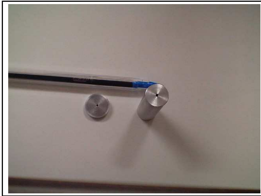
Figure 4.15: The bottom and middle centres used for alignment of the output optical system.
