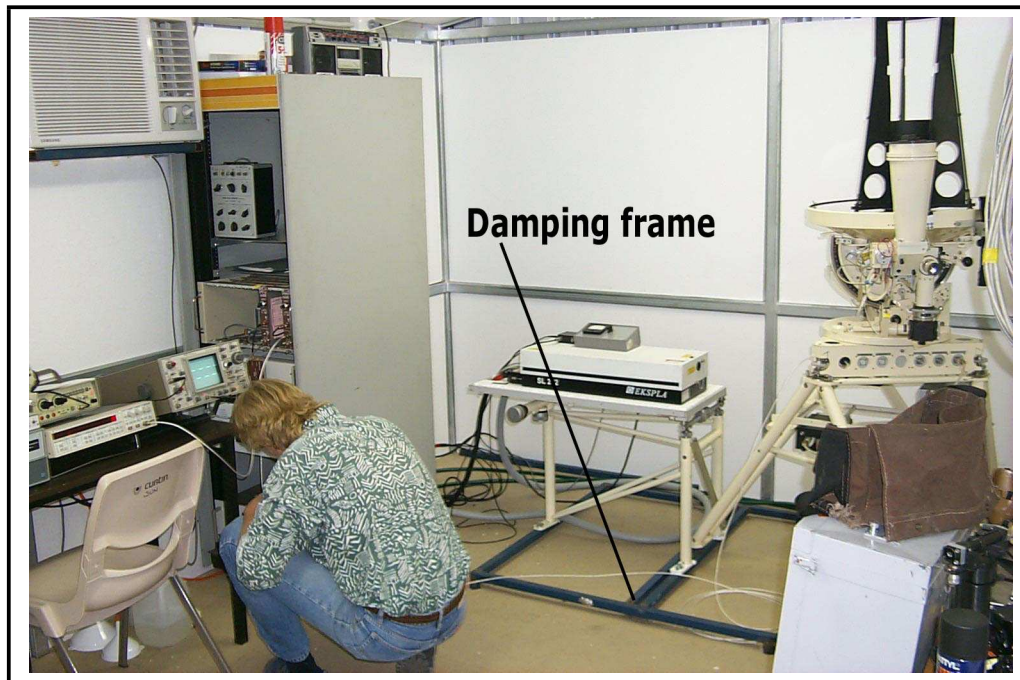
Figure 5.1: PSLR equipment layout in the roof top test facility. The blue vibration damping frame is visible just above the floor of the facility.
