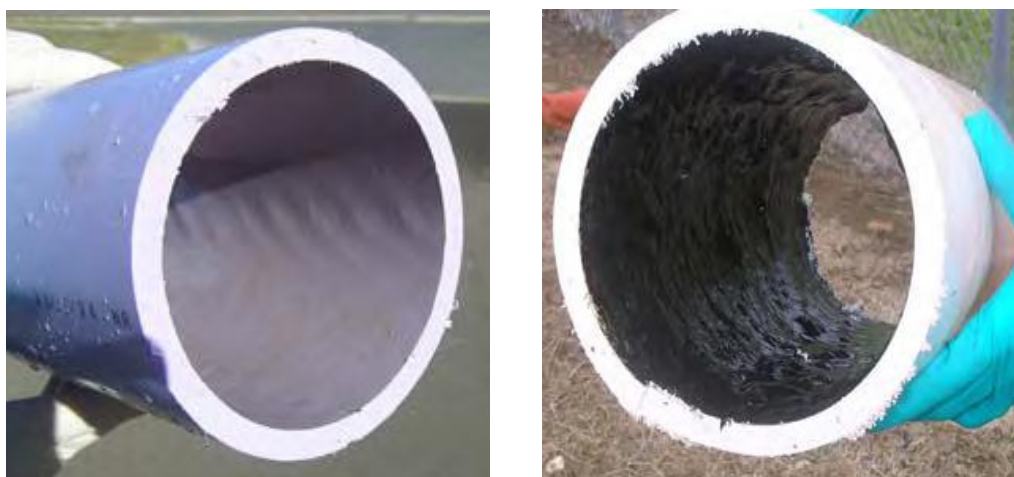
Figure 3.4 Photos of biofilms from left, Site A tertiary treated recycled water (Biofilm 12) and right, Site C secondary treated recycled water (Biofilm 150). Photos from Storey & Kaucner (2009).
