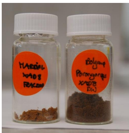
Figure 5.7 Photograph of HPO fractions isolated from Harding Dam and Bolganup Creek - higher yield of Bolganup is evident.
