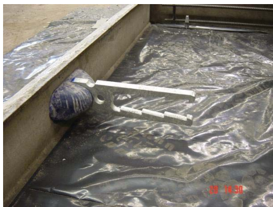
(a) Series 1 anchor with no reinforcement
