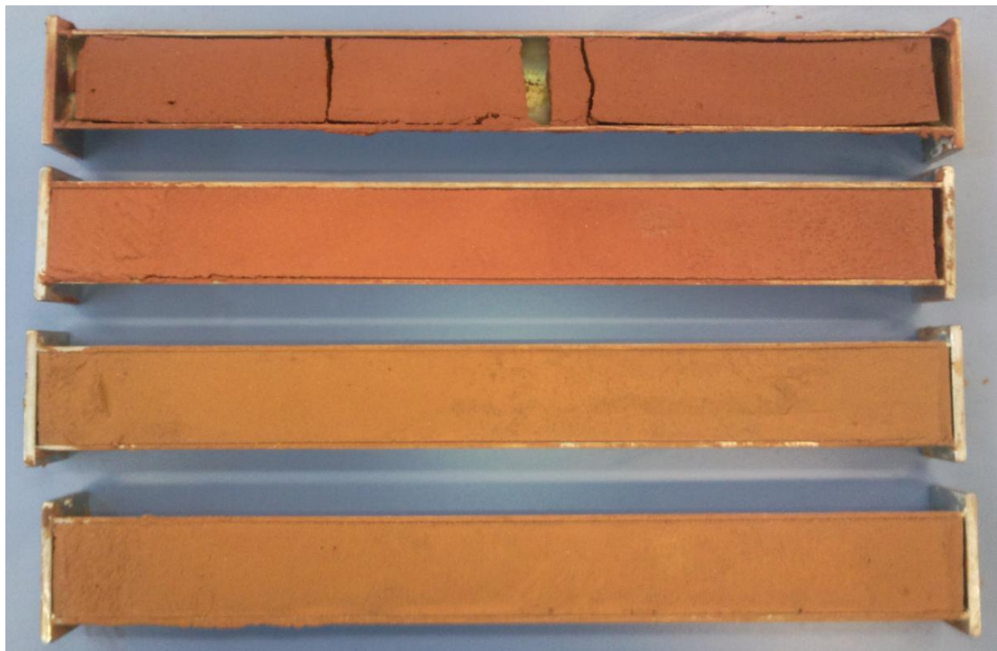
Figure 3.5: Photograph of dried moulds for linear shrinkage test
