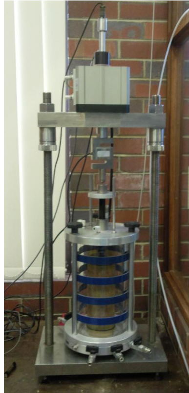
Figure 3.7: Photograph of tri-axial apparatus used for resilient modulus testing
