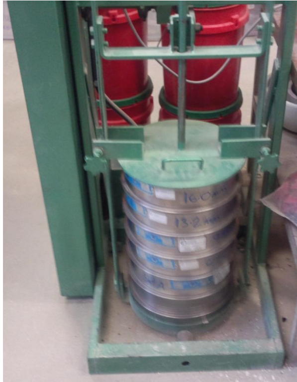
Figure 3.2: Photograph of mechanical agitator used for large sieves
