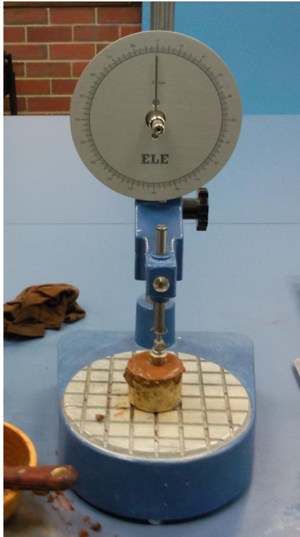
Figure 3.4: Photograph of cone penetrometer setup
