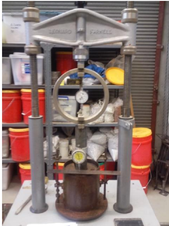
Figure 3.6: Photograph of the apparatus and setup for CBR penetration testing
