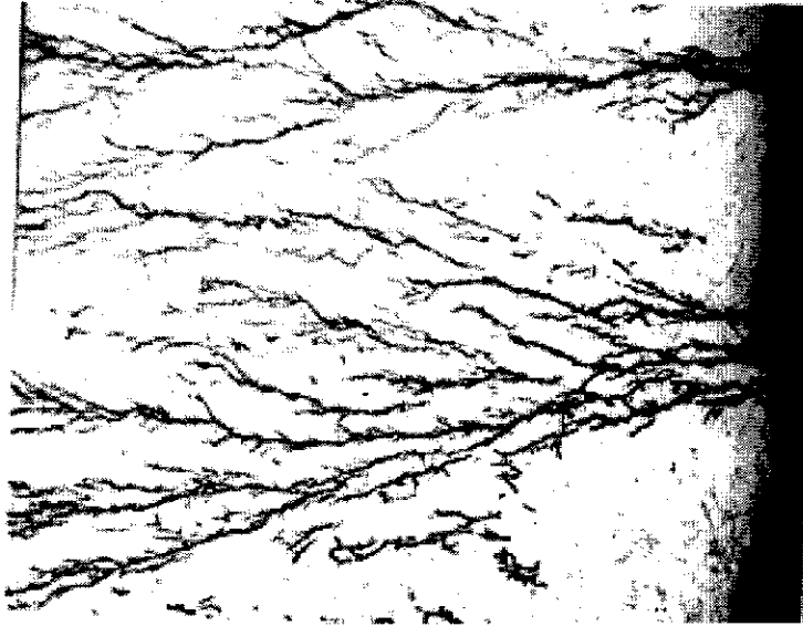
Figure 2.3: Stress corrosion cracking of stainless steel [30].
