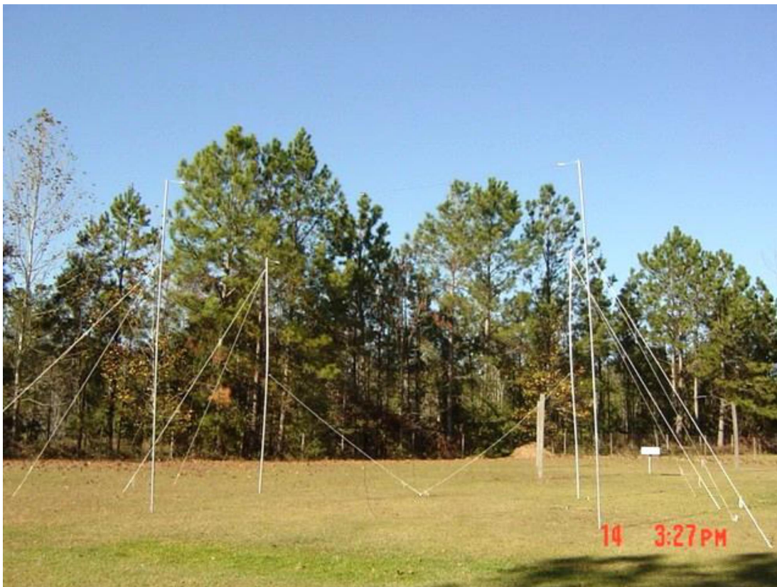
Figure 2.2: Radio JOVE dual dipole antenna, Figure 7.3c from the Radio JOVE Antenna Manual. This picture shows the different guying arrangements for metal (foreground) and PVC masts.
