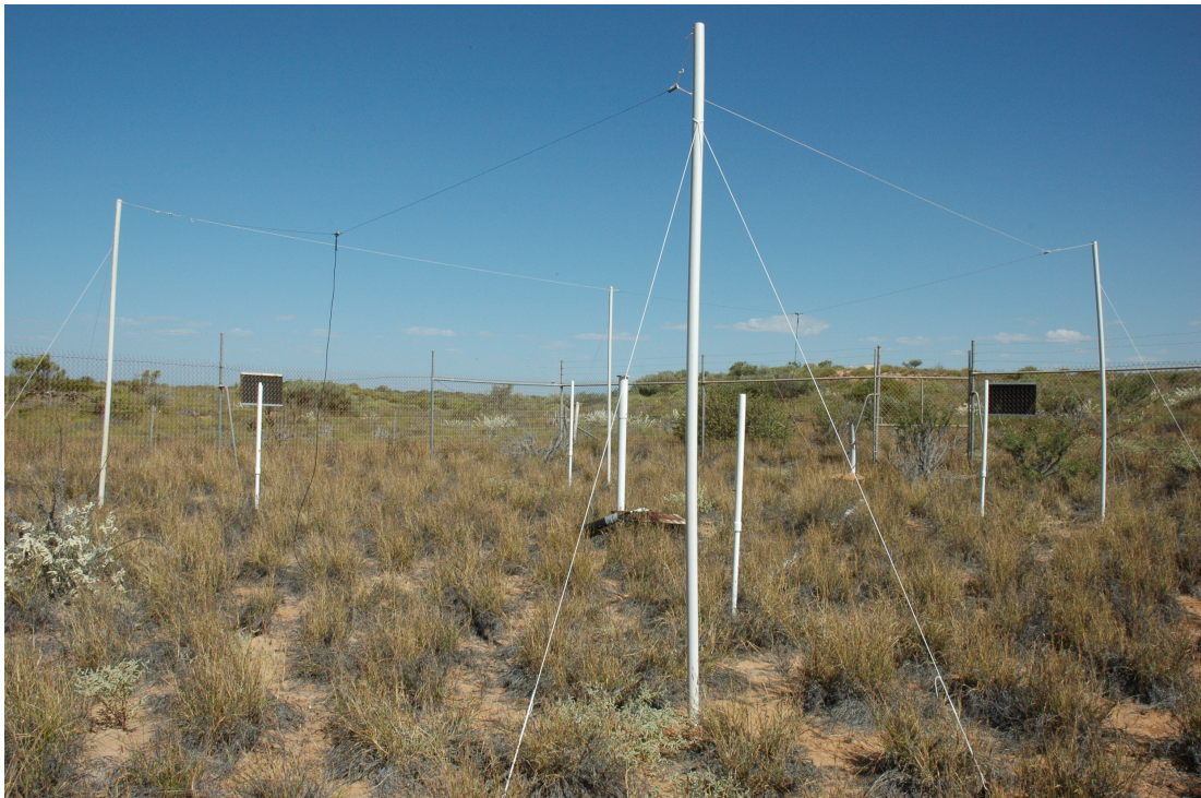
Figure 4.14: LSO 20 MHz Antenna on 14 th October 2010. The short white poles are all that remains of a previous antenna destroyed by cyclone Vance.
