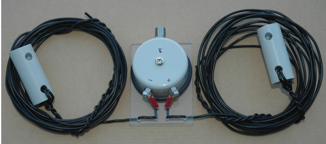
Figure 4.8: Gingin 17 MHz Dipole assembly. The clear acrylic backing of the balun assembly provides strain relief for the dipole wires and weather protection using a rubber gasket.
