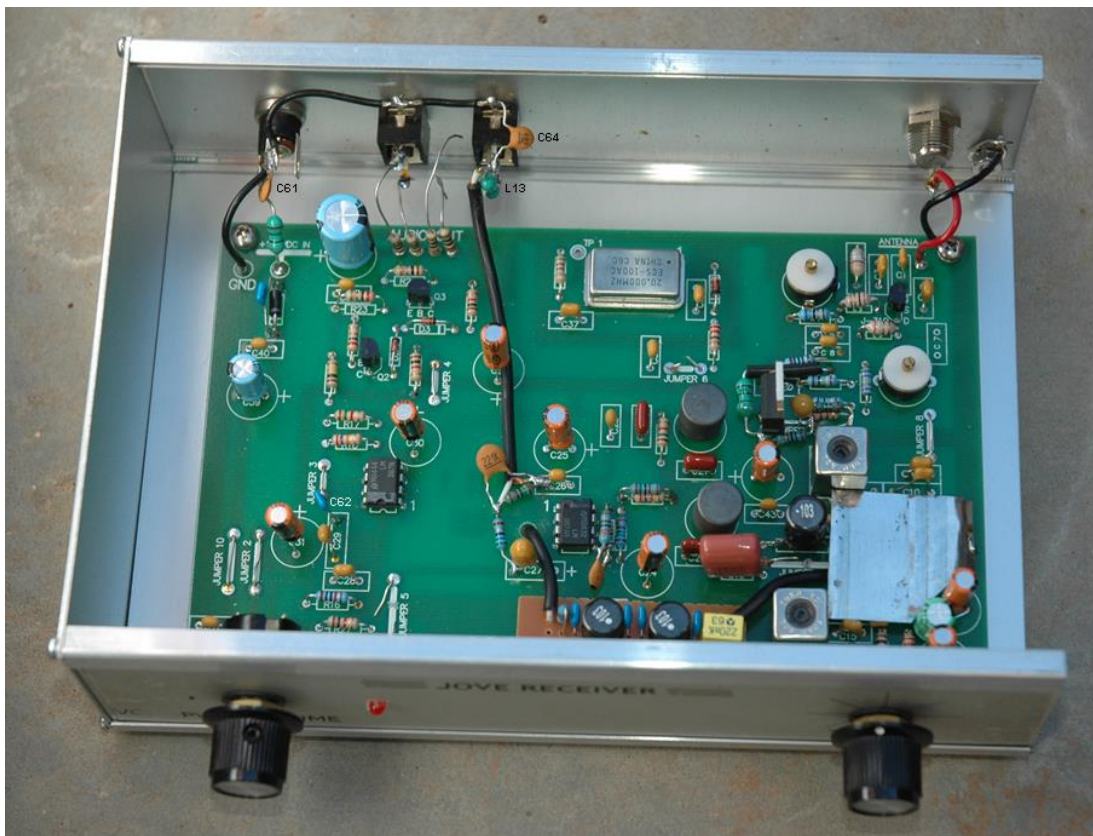
Figure 4.15: LSO modified 20.1 MHz JOVE Receiver showing additional components C61, C62, C64 and L13.
