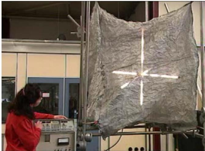
**Figure 1-14:** The Vibrating Intrinsic Reverberation Chamber: VIRC (no need for a stirrer) [36].
