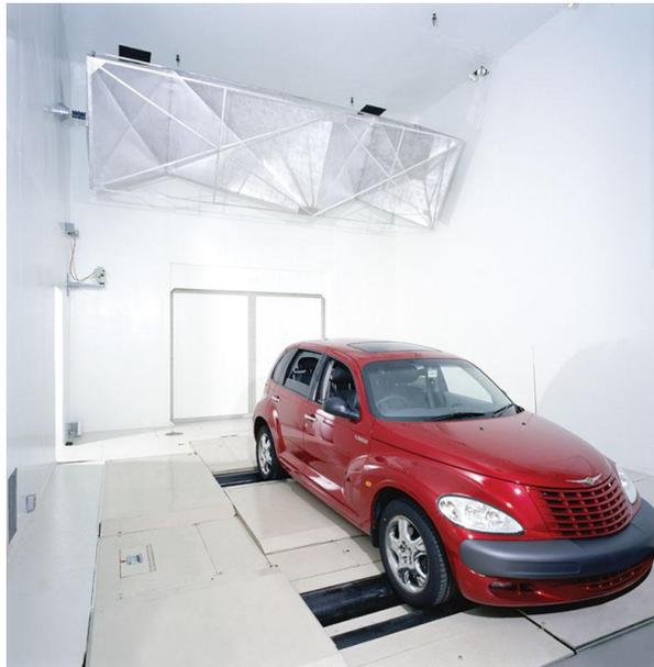
**Figure 1-1:** Smart 80 RC, ETS-LINDGREN, 80 MHz-18 GHz,  $\approx 7 \text{ m} \times 15 \text{ m} \times 8 \text{ m}$ .
