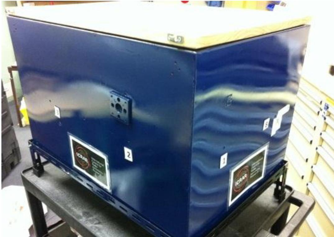
**Figure 3-10:** Scaled Model (1:5) of the CIRA Shielded Room.
