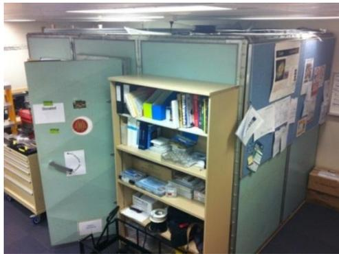
**Figure 3-1:** CIRA shielded room (3.6 m by 2.4 m by 2.4 m), expected to be a RC.
