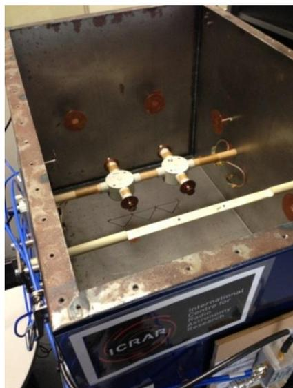
**Figure 4-11:** The Scaled Model without stirrer—this can be called a Source Stirring Reverberation Chamber (SSRC) [35].
