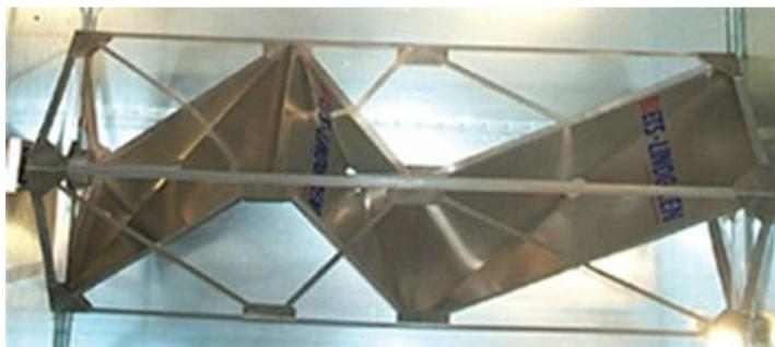
**Figure 2-12:** Z-Stirrer, ETS-LINDGREN, 1.5 m x 1.5 m x 7 m, for 80 MHz and above.
