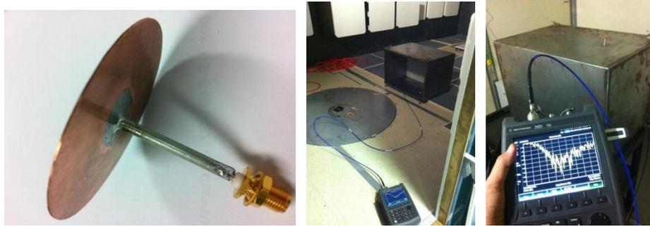
**Figure 3-12:** A top-loaded monopole specifically designed for the 1:5 Scaled Model.
