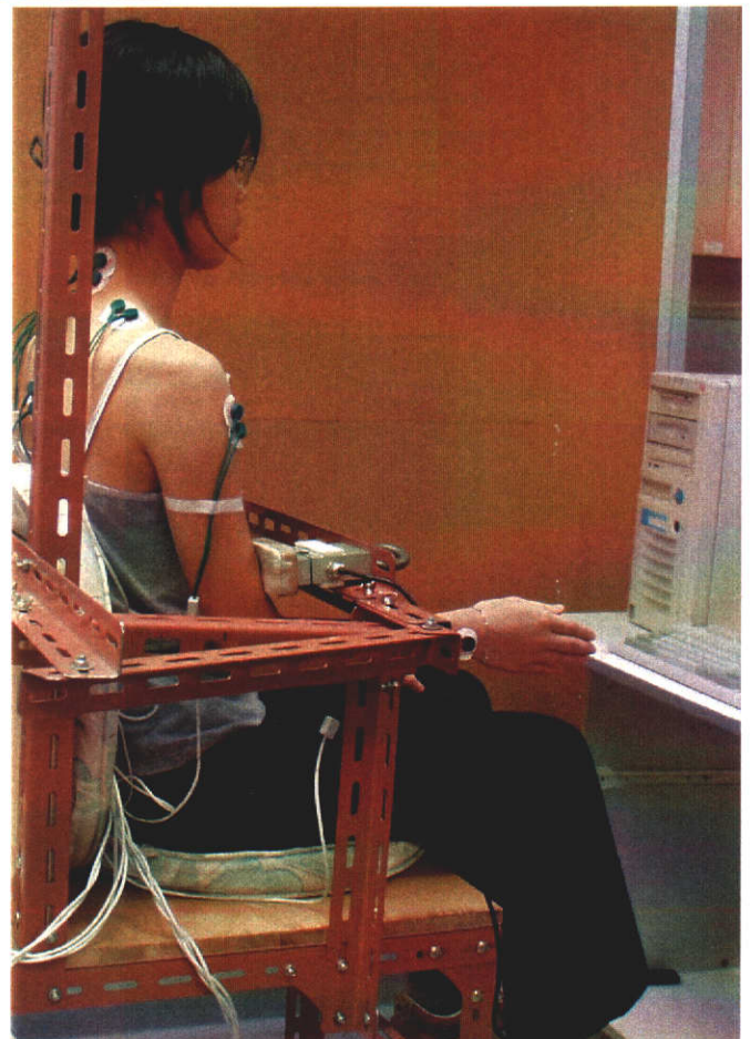
Fig. 2.5: Photograph showing a subject performing a forward flexion of the right upper arm for recording MVC of the right AD muscle
