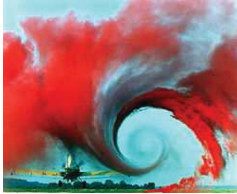
Figure 1.3 Vortex Created by the Passage of an Aircraft Wing, revealed by Colored smoke
