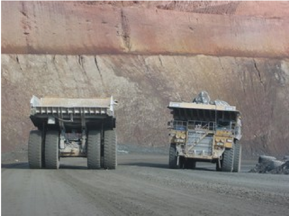
FIGURE 1.5: Large capacity mining trucks: one travelling empty down the ramp while the other travels full up the ramp (KCGM 2007b).
