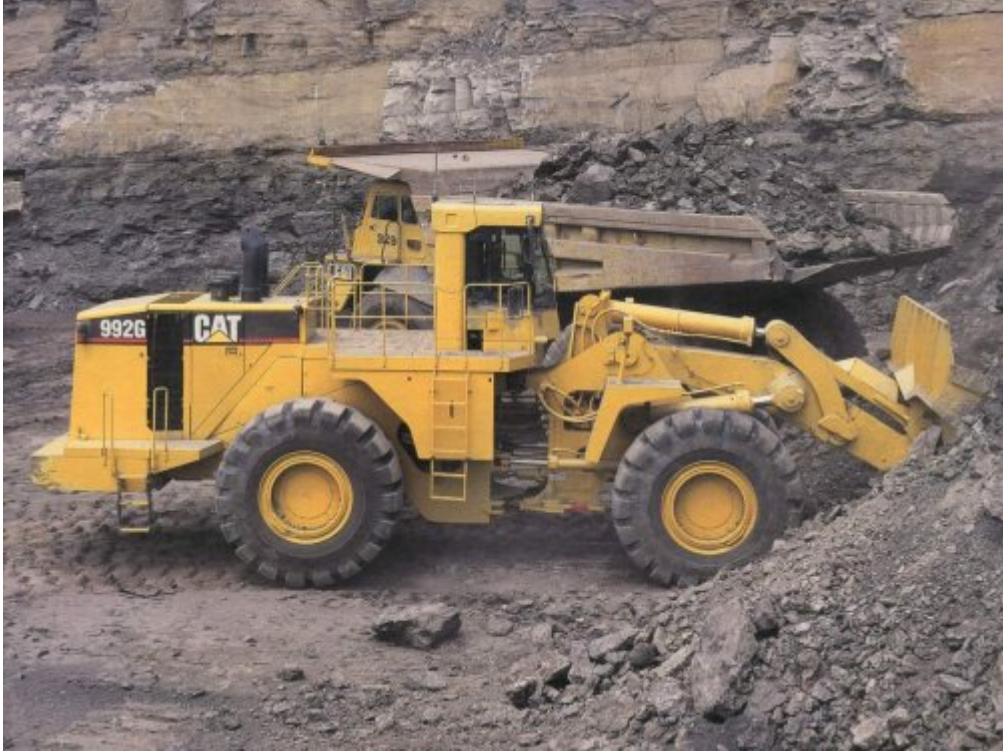
FIGURE 1.4: A CAT 992G front-end loader operating in a mine in Russia (Karelia Government 2007).
