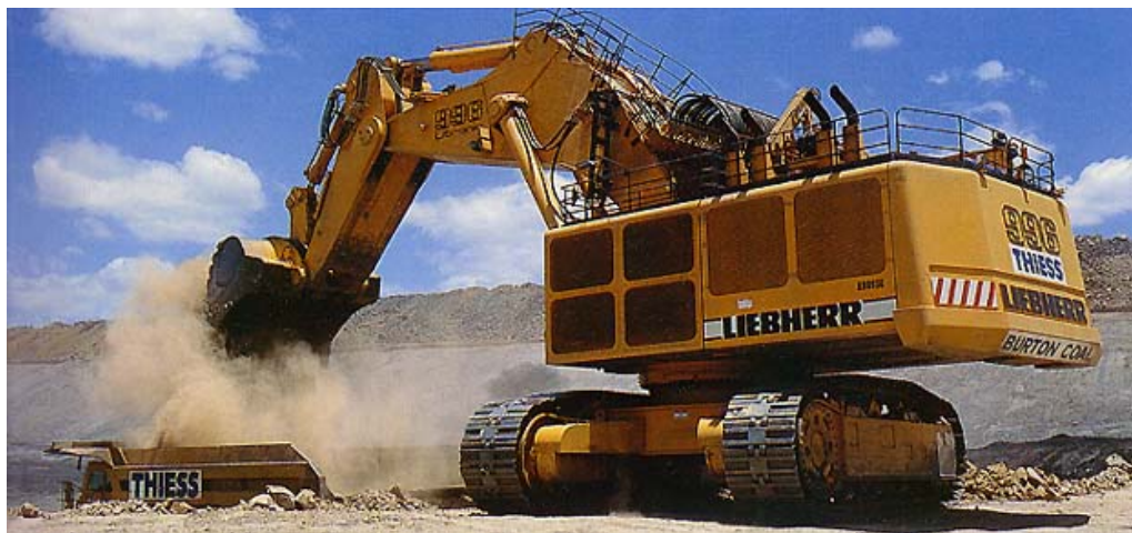
FIGURE 1.3: A Liebherr R996 hydraulic backhoe excavator (Mining-Technology 2007 a ).
