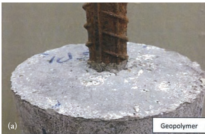
Figure 7: Corrosion of steel bar in (a) geopolymer concrete and (b) ordinary concrete.
