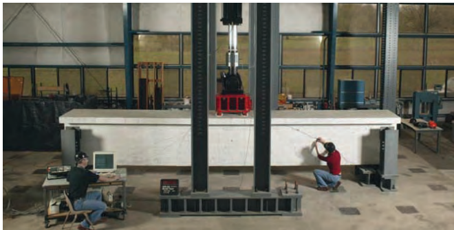
Figure 12: Large bridge girders predicted response and observed response.
