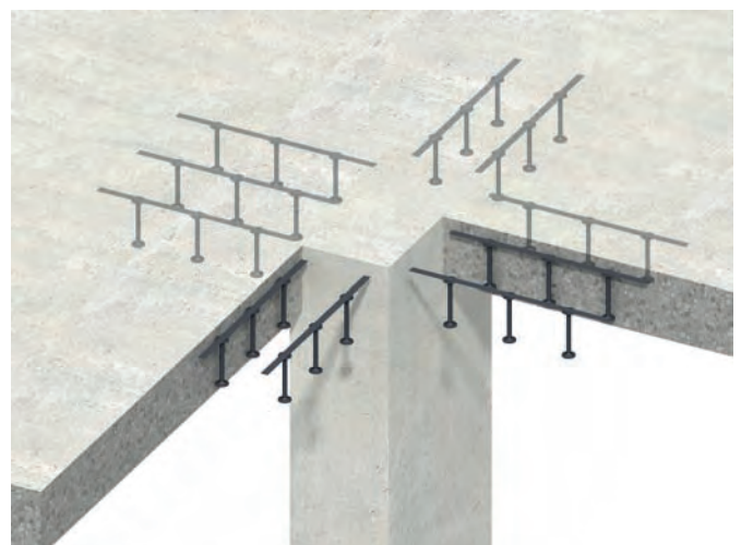
Figure 2: Shear rails arranged around a column head.
