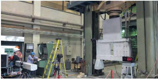
Figure 13: Testing one-fifth scale model of transfer girder.
