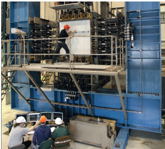
Figure 8: Shell element tester with 60 computer controlled actuators.
