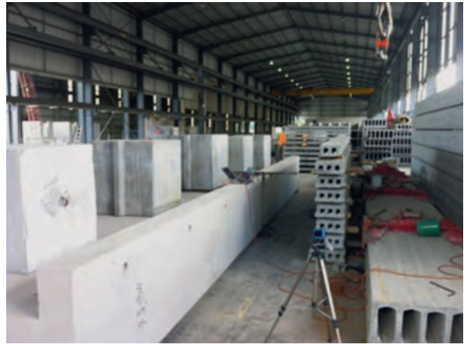
Figure 5: Full scale load test at Precast factory.
