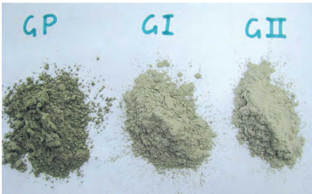
Figure 1: Colour comparison of binders: GP (General purpose OPC), GI (Geopolymer 1) and GII (Geopolymer 2).
