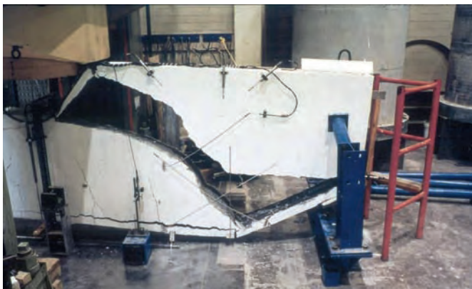
Figure 1: Failure of slab strip without shear reinforcement 1 .
