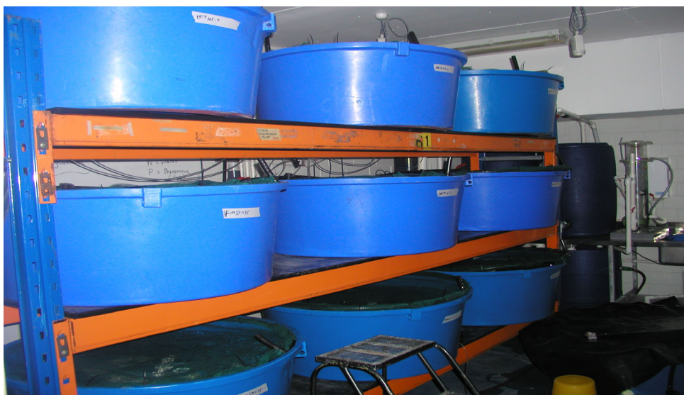
Plate 3.3 Nine x 300L tanks in recirculation system
