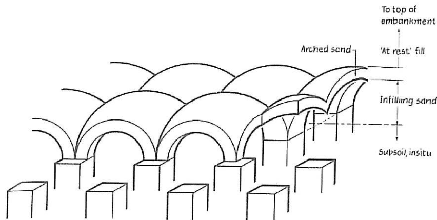
Figure 2: Isometric view of a grid of columns and a series of domes forming vaults spanning between them (Hewlett and Randolph, 1988)
