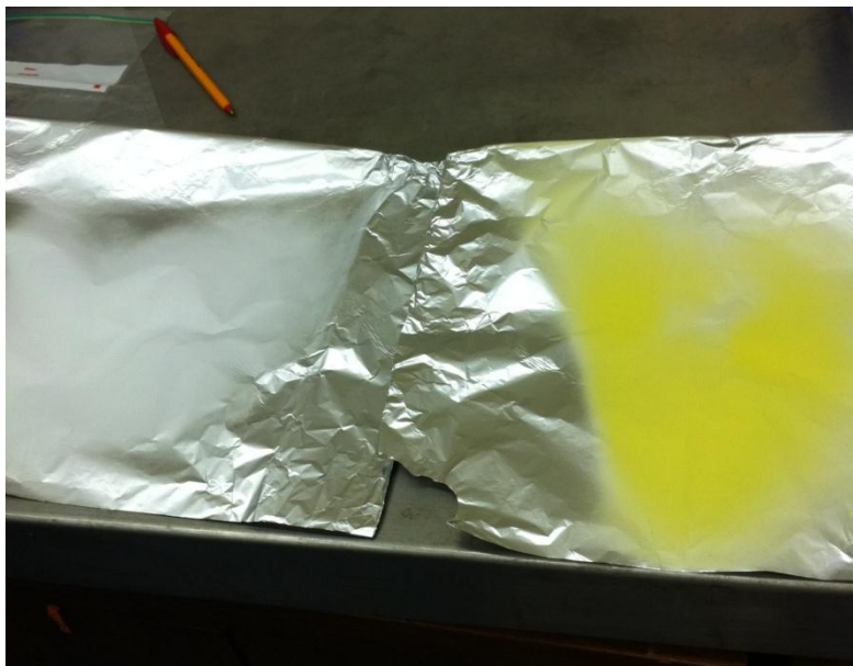
Figure 8.6: Final product collected on the aluminium foil after the process was completed. The product on the left side is the control PLA nanofibre mat; while at the right side is the Bi 2 O 3 /PLA nanofibre mat.
