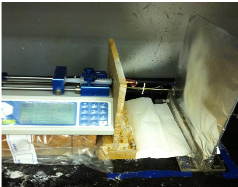
Figure 8.5: Electrospinning experimental set up to perform the electrospinning process.
