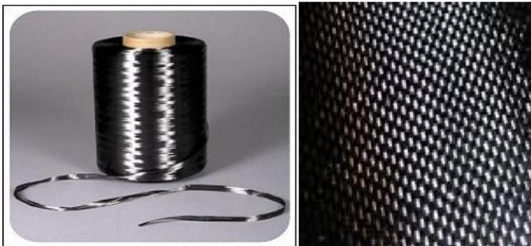
Figure 2.16: Carbon fibres (Singh, 2011).
