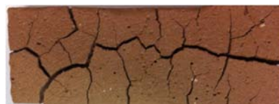
Fig. 5 Photograph of the geopolymer composites loaded with 0 wt% CF after heating at 1000 °C.
