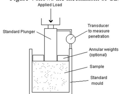
Figure. 4 Mechanism of CBR Test Machine( Gray,1983)
