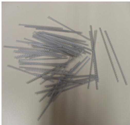
Fig. 3 Plastic fibre
