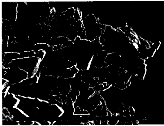
Figure 9.6 FESEM images of COM crystals grown for thirteen hours in an aqueous solution of PT: (a) whole and fractured crystals, (b) exposed edge of a fractured crystal.
