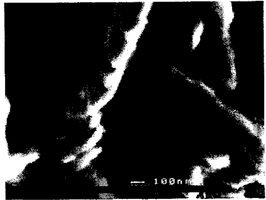
Figure 9.5 FESEM images of COM crystals grown for one hour in an aqueous solution of PT: (a) whole crystals, (b) fractured crystals at higher magnification.
