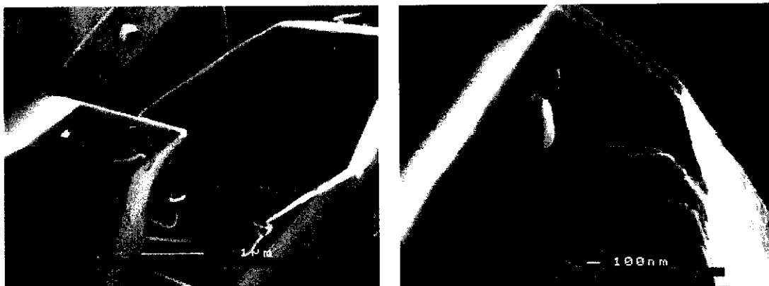
Figure 9.2 FESEM images of COM crystals grown in distilled water for thirteen hours then treated with Proteinase K: (a) whole crystals, (b) exposed internal surface of fractured crystal.
