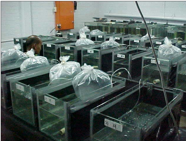
Plate 5.1 Experimental glass aquaria (54L, filled to 25L), showing fish bags.
