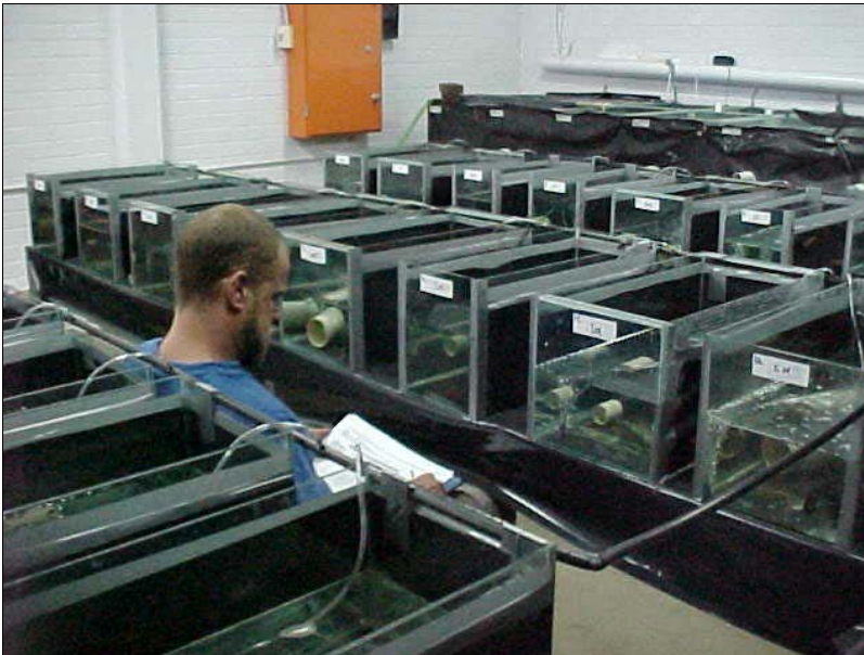
Plate 4.1 Experimental systems, 54L glass aquaria - filled to 25L
