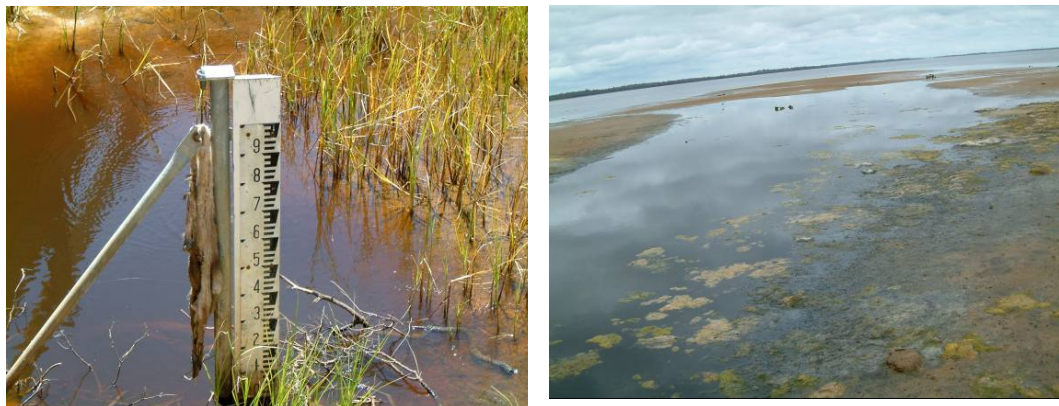
Figure 3-19: Backwater Height gauge at the End of Fauntleroy Drain (near Peel Inlet)
