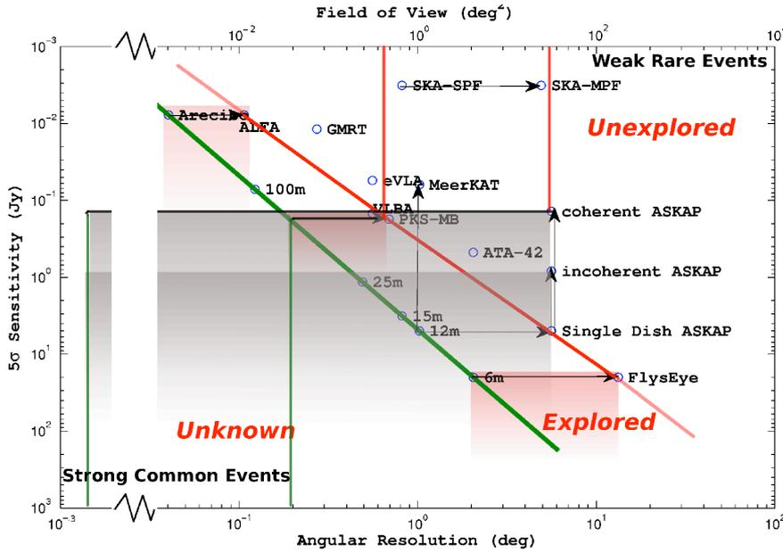
Figure 1: The CRAFT survey will search a greater area of parameter space than other similar surveys. The parameter space searched by the Arcibo-ALFA, Parkes-MB and ATA-FlyEye surveys are indicated with orange boxes. These are bound between the green line, the single dish resolution and the red line, the FoV with a multi-beam instrument. CRAFT has wide FoV and high resolution as indicated by the gray area. This is an essential pre-requisite for the identification of a transient source.
