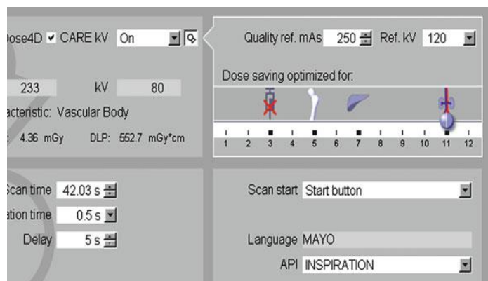
Figure 2.2 Example of using automatic software to select the optimal tube voltage and to prescribe the dose-reduced technique (CARE kV, Siemens Healthcare). The reference technique was at 120 kV and 250 quality reference mAs. The slider bar position, which corresponds to a strength setting, was at 11. 80 kV was identified as the optimal tube voltage [1]
