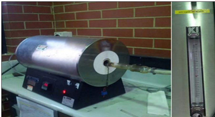
Figure 3.7 Horizontal Tube furnace used in the preparation of biomass based activated carbon
