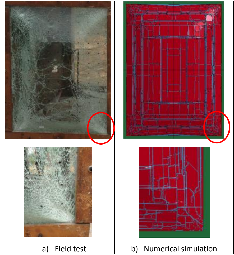
Figure 13 Comparison of failure patterns for pane 1-1-1
