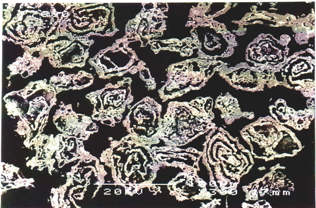
Figure 5.27c BSE micrograph of iron-rich pentlandite collected at 680°C. The oxide has formed concentric layers.
