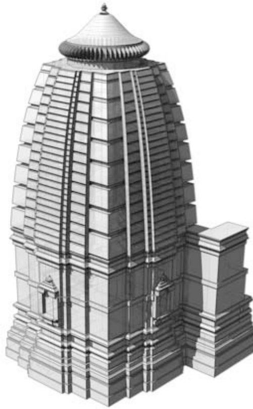
Figure 2. 3D reconstruction of the Temple of Ranakdevi, Wadhwan. The superstructure geometry is modelled using the geometric progression for scaling and curvature of individual units.
